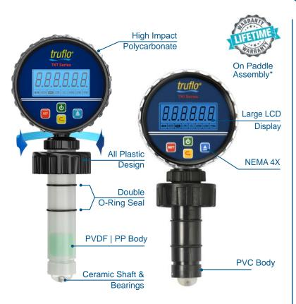
Simple to install with time-honored reliable performance, Truflo TIB Series Paddlewheel Flow Sensors are highly repeatable, rugged sensors that offer exceptional value with little or no maintenance. The TIB Series has a process-ready open collector signal with a wide dynamic flow range of 0.1 to 6 m/s (0.3 to 20 ft/s). The sensor measures liquid flow rates in full pipes and can be used in low pressure systems.
